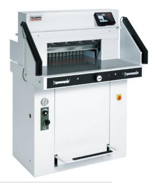
Comprehensive SCS safety package: patented EASY CUT electronic blade activation bars for true two-hand operation; IR light beam safety curtain on front table; safety cover on rear table; lockable main switch; 24 volt controls (low voltage); patented IDEAL safety drive; automatic blade and clamp return from every position; blade changing device covers cutting edge of blade; blade depth adjustment from outside of machine; blade and cutting stick can be changed without removing covers.
