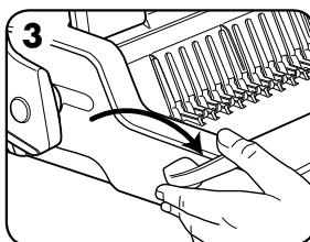
3. Pull comb-opening lever forward to open the comb.
