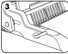
3. Load punched sheets directly onto the opened comb. Starting with the front of the document.
