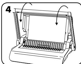
4. Test punch scrap sheets to check edge guide setting.
