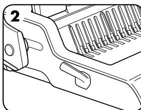
2. Insert the plastic comb into the mechanism.
