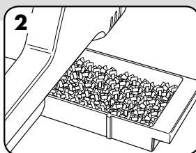
2. Check waste tray is empty and correctly fitted.
