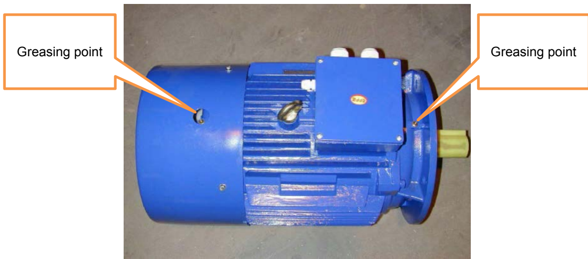
Figure 7-1 – Greasing point electric motors
