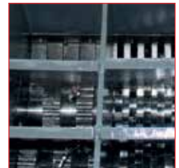
Dual HDD/SSD cutter heads accessed via dual feed slots
