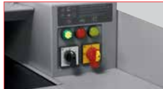
Easy to use controls with lockout switch
