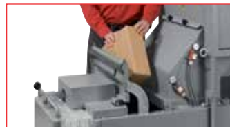
Separate cardboard feed chamber on 14.87 Series
