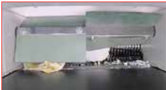
Infeed conveyor with paddle system
