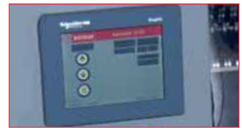
SmartShred PLC Based Touchscreen Control Interface
