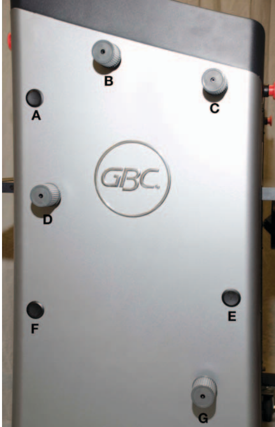
Figure 26. Tension Knobs on end of the laminator.
