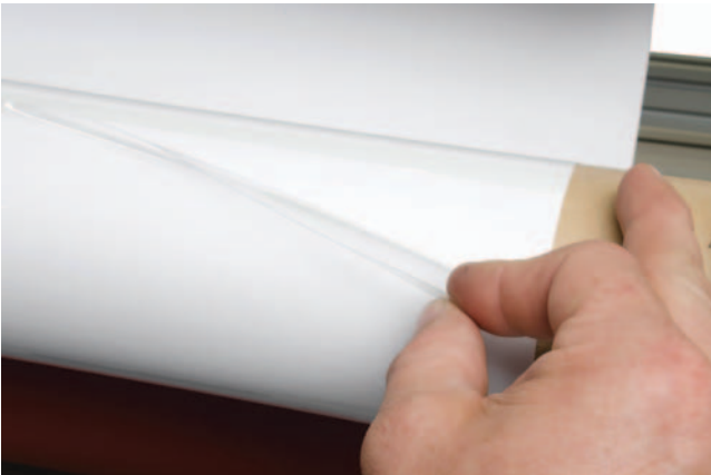
Figure 39. Separating film from the release liner.
