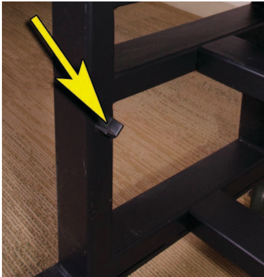
Figure 13. Shaft Storage Cradle on Back of the Laminator.
