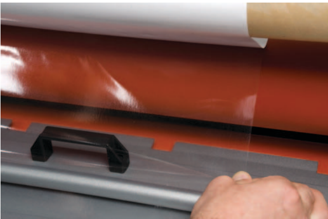
Figure 40. Pulling laminate film to Upper Main Roller.
