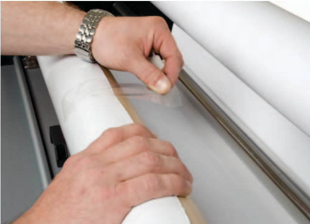
Figure 38. Taping film to the rewind tube.
