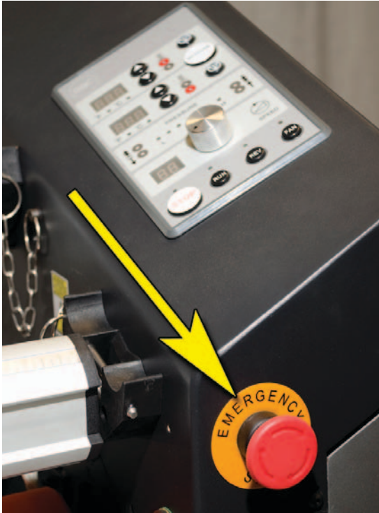
Figure 5. Emergency Stop Switch near Operator Panel.
