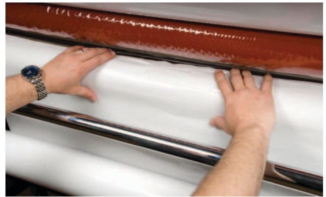
Figure 41. Attaching mounting adhesive (on bottom) to the PSA.
