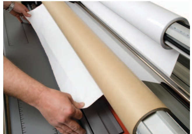
Figure 37. Pulling pressure sensitive adhesive (PSA) film to the Rewind Tube.
