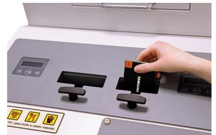
Fig. 5b 2.5" Feed Chamber
