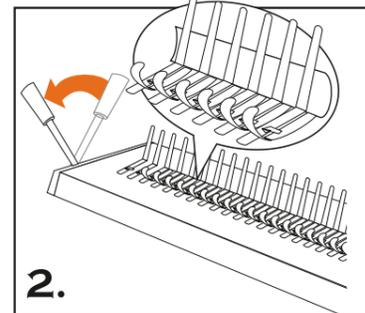
**IMPORTANT:** Depending on the size of the comb used, it may not be necessary to pull the Comb Opener Handle all the way down.
