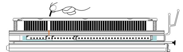
3. Re-Install the punch pin retainer cover onto the die set. Make sure both sides of the retainer cover are securely locked in place.
