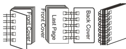
The seam of a well closed wire should have the narrow loop just touching the wide loop. If this is not the case on your first try, slightly adjust the Wire Closer Control towards the LEFT (for the under-closed wire) or the RIGHT (for the over-closed wire), so the next wire you close would have a perfect closure seam.
