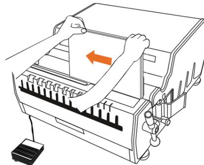
4. Activate the punching action by stepping on the Foot Pedal or by pressing the **Manual Punch Switch** on Manual Control Panel.
