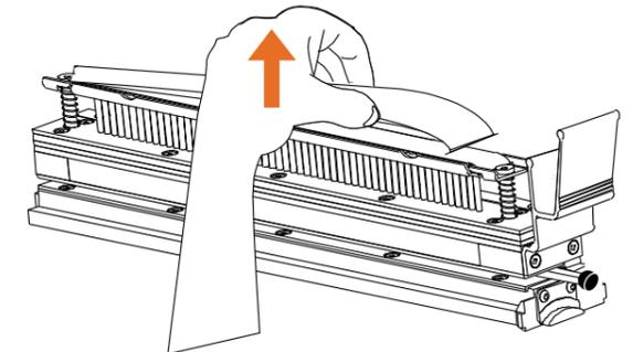
2. Remove the desired punch pin from the die set.
