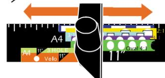
3. Insert sheets into the Punch Throat from right-hand side of the machine, then slide it towards the left until it aligns to the Side Margin Control.
