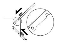
Insert the 1st fold plate(long plate) into the studs (A) and (B) and lock into position.
