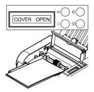
The machine cover must be closed.
