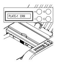
Mount the 1st fold plate according to instruction. See "Installation".
