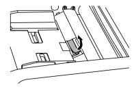
Remove the separator with a sharp edged tool and replace them.
