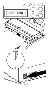
Switch off the machine and wait 1min before switching on again.
