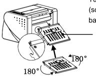
Turn the 2nd fold plate 180 degrees (script is in reversed position) and put back into the machine.
