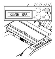
Press the "C" button to clear up the malfunctions.
