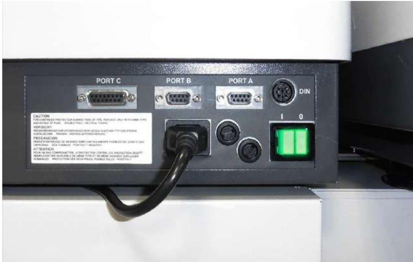
Figure 2.1 - Rear I/O toggle switch
